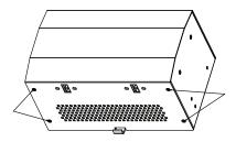
**3.** Carefully slide the front cover forward and off the enclosure. Do not disconnect the wires from the polarized terminals.
