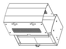
10. Secure the assembly with eight screws.
