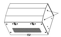
2. Remove eight screws from the top and bottom sides of the enclosure.
