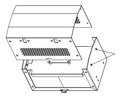
9. Slide the front cover onto the enclosure.
