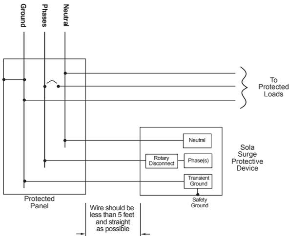
**Wire Sizing:** With parallel connection, the size of the wiring to the SPD unit is independent of the protected circuit's ampacity. For suggested wire size, refer to the "Individual Product Sheet".
