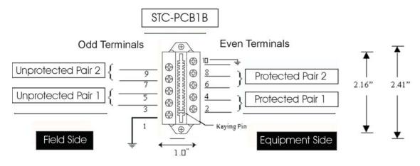
Ground Terminal 1 or 10 (internally tied together) to building approved ground. The STC-PCB1B accommodates 24 to 10 AWG wire.
