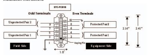
Ground Terminal 1 or 10 (internally tied together) to building approved ground. STC-PCB1B accommodates 24 to 10 AWG wires.
